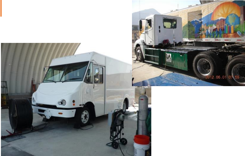
Dynamometer Systems capable of testing a wide range of electric-drive vehicles
